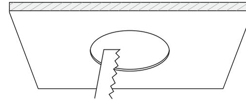
To maintain IP65 rating on XDF35, ensure that the luminaire is installed on a flat, level ceiling and that the luminaire has an adequate seal to the mounting surface.
