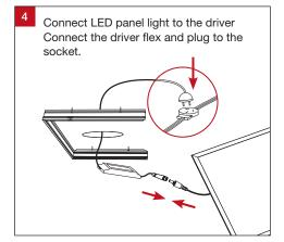
Slide the LED panel light with the driver into the surface mounted frame. Re-screw the removed side panel back to secure the panel.
