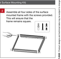
Install the surface mounted frame to the ceiling (A) with all four sides attached.
